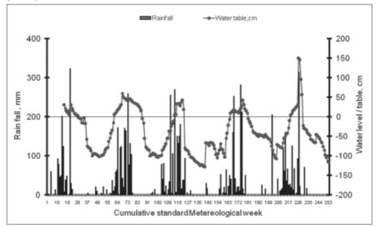
**Fig. 2.** The changes in level of water inside observation bore during experimental period and weekly rainfall underneath *Casuarina* vegetation at Patna from 2004-05 to 2009-10 (March).
