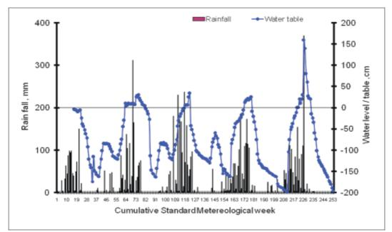
**Fig. 1.** The changes in level of water inside observation bore during experimental period and weekly rainfall underneath *Casuarina* vegetation at Baghadi from 2004-05 to 2009-10 (March).
