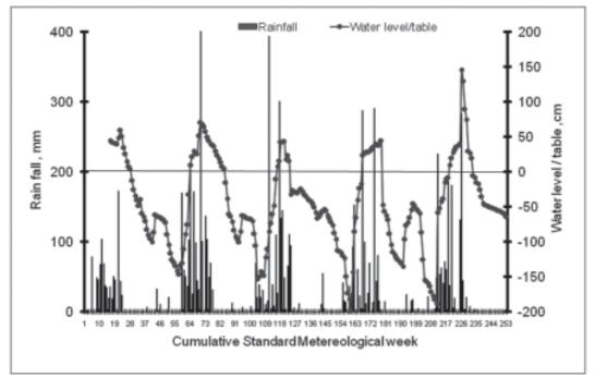
**Fig. 4** The changes in level of water inside observation bore during experimental period and weekly rainfall underneath *Eucalyptus* vegetation at Ambapada from 2004-05 to 2009-10 (March).
