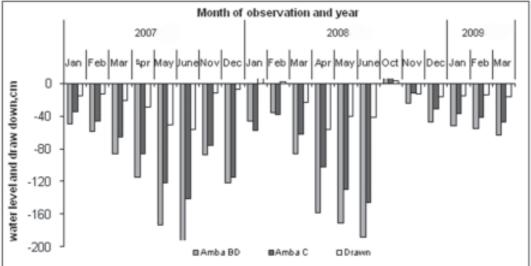
**Fig. 6.** The monthly changes in water level in observation bore well inside *Eucalyptus* plantation (BD) and in observation bore well out side plantation (C) and the difference in water level (BD-C, Drawn) at Alisibindha and Ambapada .
