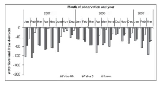
**Fig. 5.** The monthly changes in water level in observation bore well inside *Casuarina* plantation (BD) and in observation bore well out side plantation (C) and the difference in water level (BD-C, Drawn) at Baghadi and Patna.
