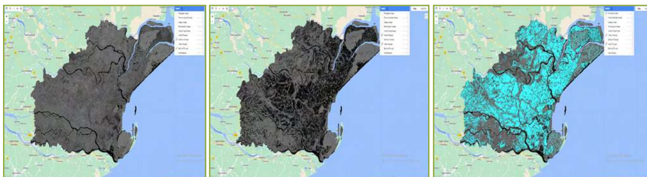
Fig. 11. Delineated Flooded area in Kendrapara (August, 2023) in GEE interface @ threshold value of 1.10
