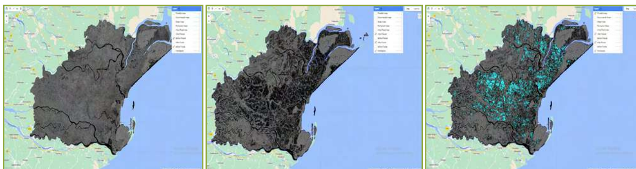
Fig. 12. Delineated Flooded area in Kendrapada (August, 2023) in GEE interface @ threshold value of 1.50
