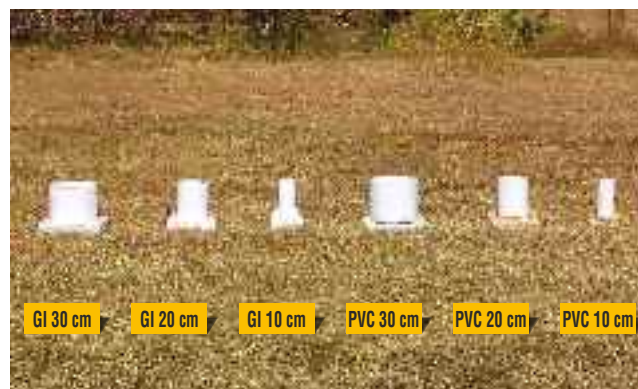
Mini-pan evaporimeters (GI and PVC) of different sizes installed research farm
