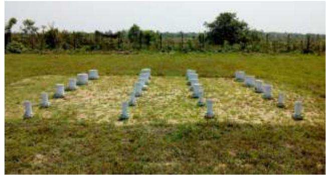
Mini pan-evaporimeters (GI and PVC) of different sizes installed at ICAR-IIWM research farm, Mendhasal
