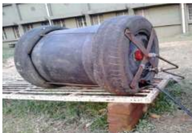
Fig. 40 Prototype (built from scrap of institute workshop) of rolling water tank on 25 cm high ramp at testing area
