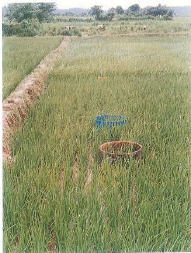
Lysimeters in the experimental plot.
