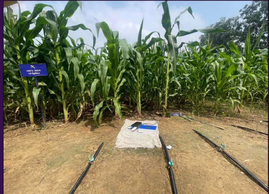
An IoT-enabled capacitance-based soil moisture sensor installed at different locations
