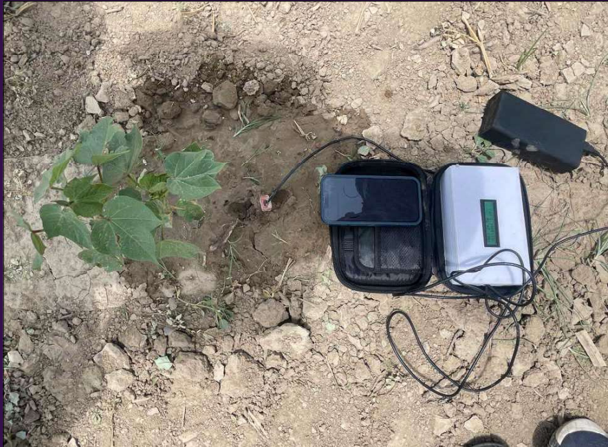
An IoT-enabled capacitance-based soil moisture sensor installed at different locations
